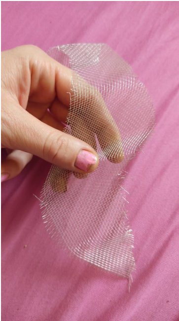
aluminium mesh (current collector)
