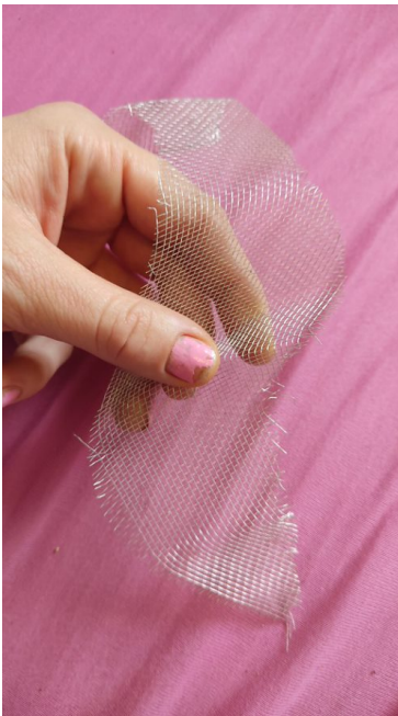
aluminium mesh (current collector)
