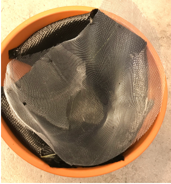
Mesh and carbon cloth wrapped inside the ceramic pot
